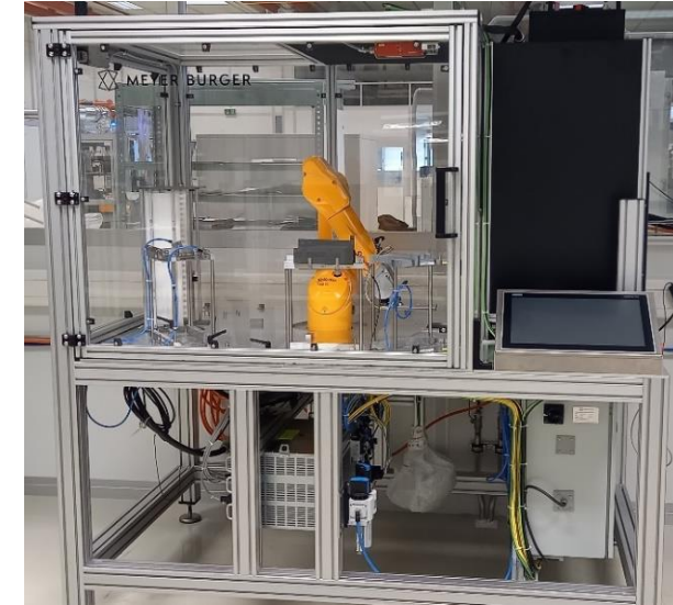
SpotLight and 6-axis robot loading/unloading & wafer / cell handling automation
